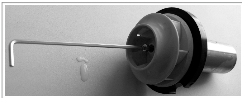
Fig. 8: Disassembly of impeller wheel
