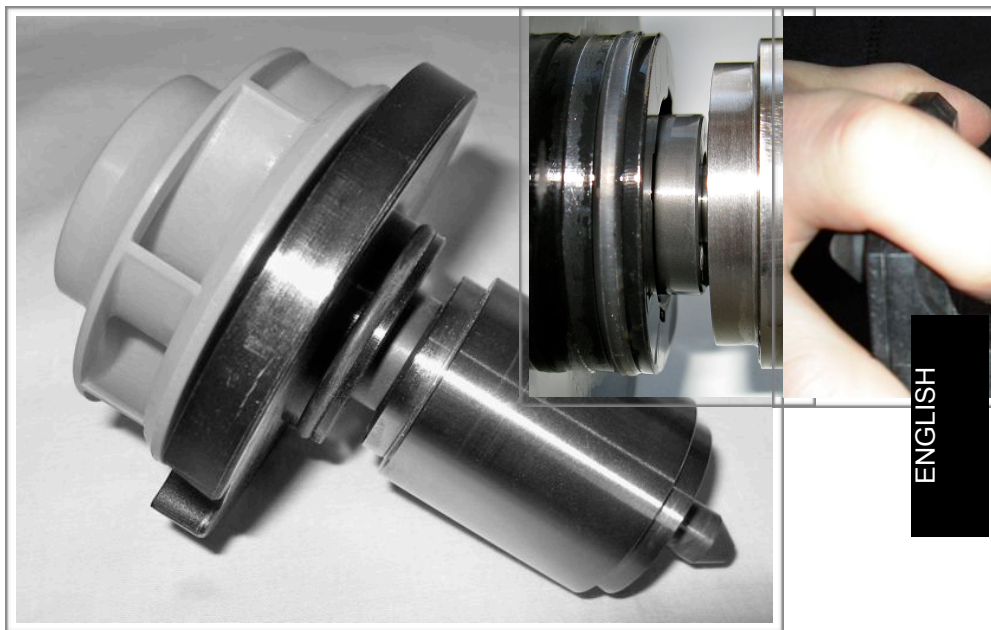
Fig. 7a/b: Removed impeller component, close-up of bearing (right)
