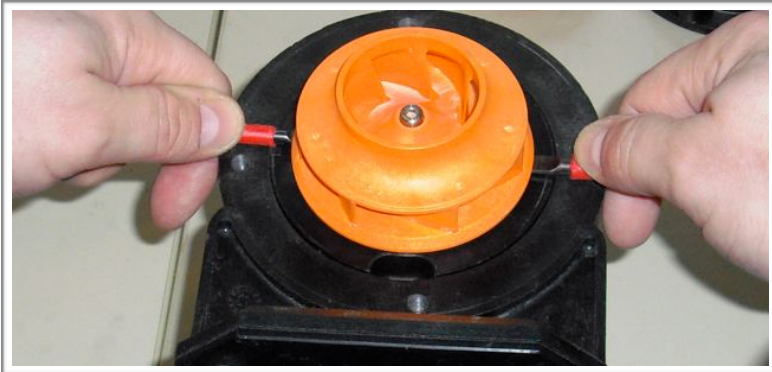
Fig. 6a: Loosening of impeller components
